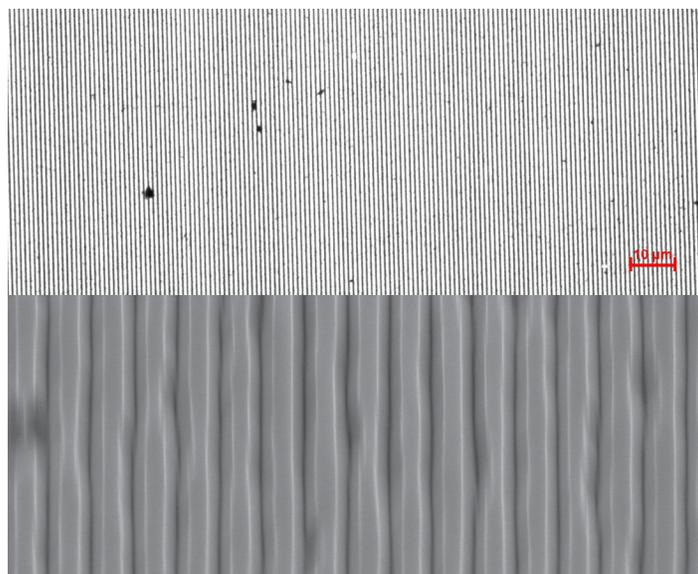
Images of MagAssemble transmission and reflection diffraction gratings. Top: Optical image of SiO<sub>2</sub> lines with a square-wave profile and 1.5 μm trench depth. Bottom: SEM image of Si grooves with a triangular profile.
