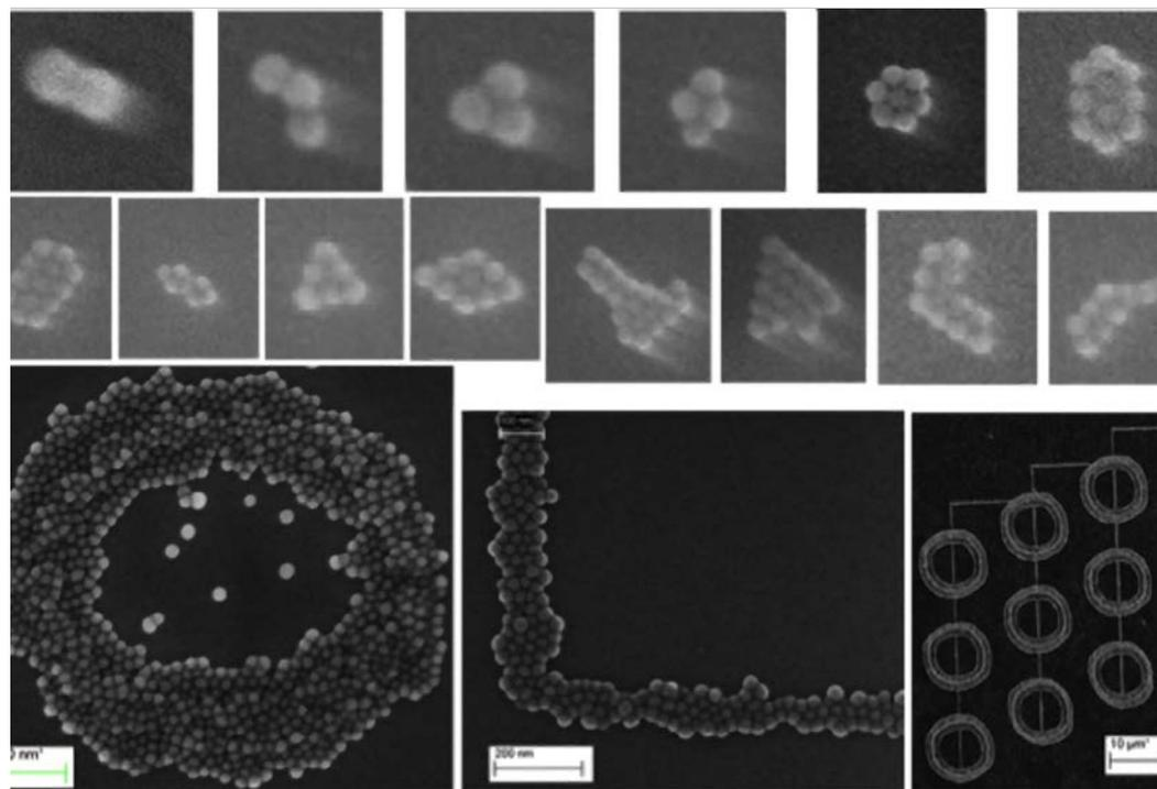
**Figure 1:** Example Scanning Electron Microscopy (SEM) images of magnetic nanoparticle self-assembly. **Top:** Random self-assembled patterns of 25 nm diameter magnetic nanoparticles. **Bottom:** Programmed assembly of nanoparticles into torii, rectangles, and more complex structures using recorded patterns on disk drive media.
