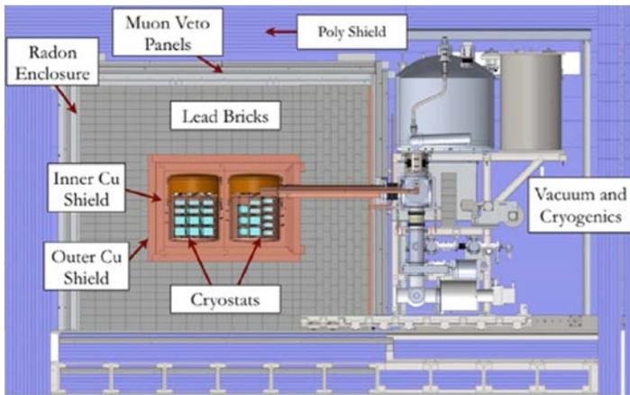
*Schematic of the Majorana Demonstrator located at the Sanford Underground Research Facility (SURF) in Lead, South Dakota. The Demonstrator holds the Germanium crystals for our search for neutrinoless double beta decay.*
