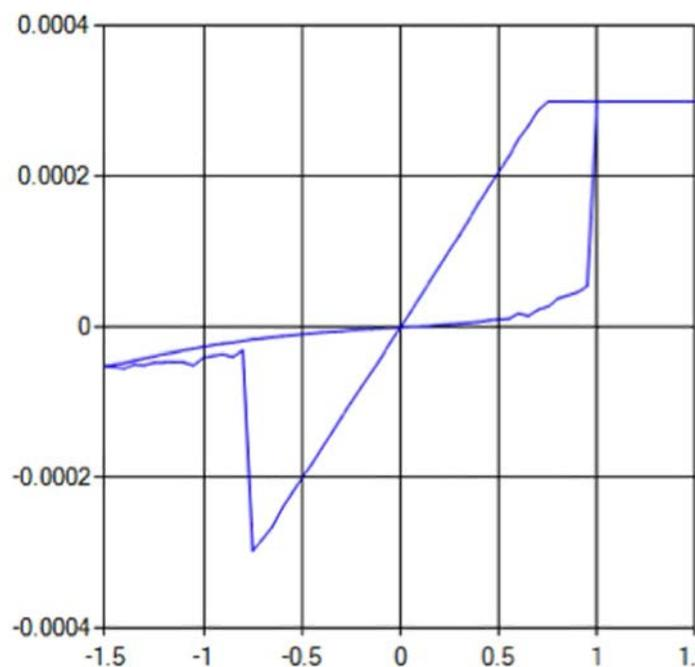
Example of I-V curve (current is in the vertical direction). The history-dependent slopes are the sign of the memory effect.
