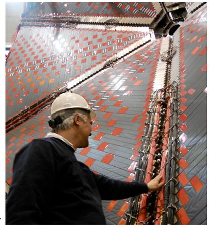
Figure 2: Dr. Gothe inspects the final implementation of our USC-built Time-of-Flight spectrometer into the CLAS12 detector at Jefferson Lab.
